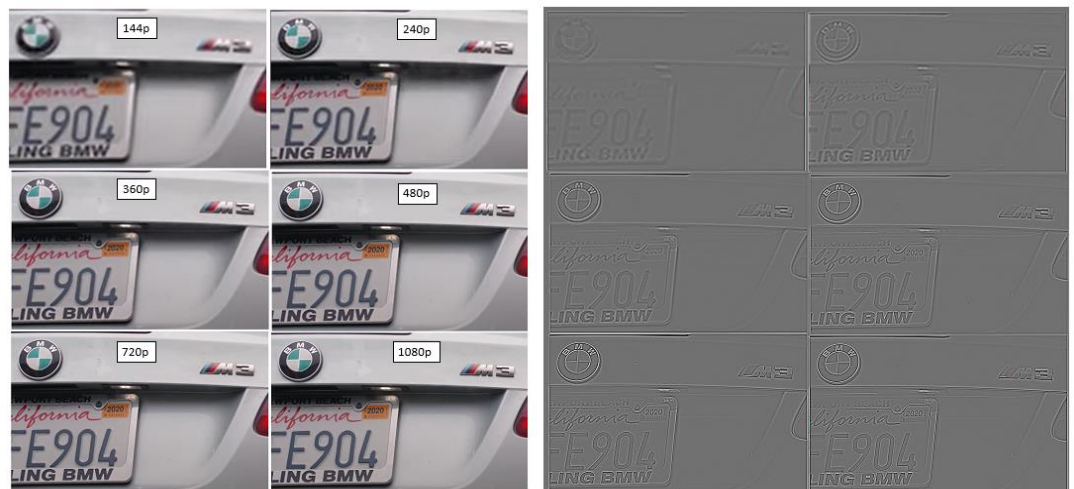
Figure 1: High pass filter yielding edge detection in the spatial domain
